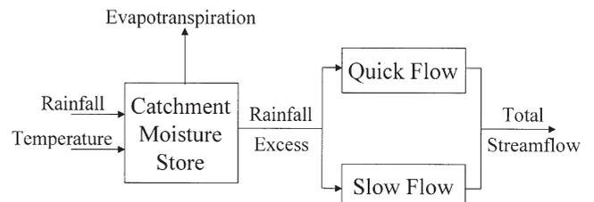
Fig. 1. Structure of the rainfall-ET-runoff model.
