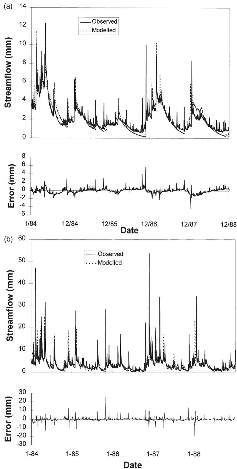
Fig. 2. (a) Simulation model fit for Coweeta Watershed 34. (b) Simulation model fit for Coweeta Watershed 36.
