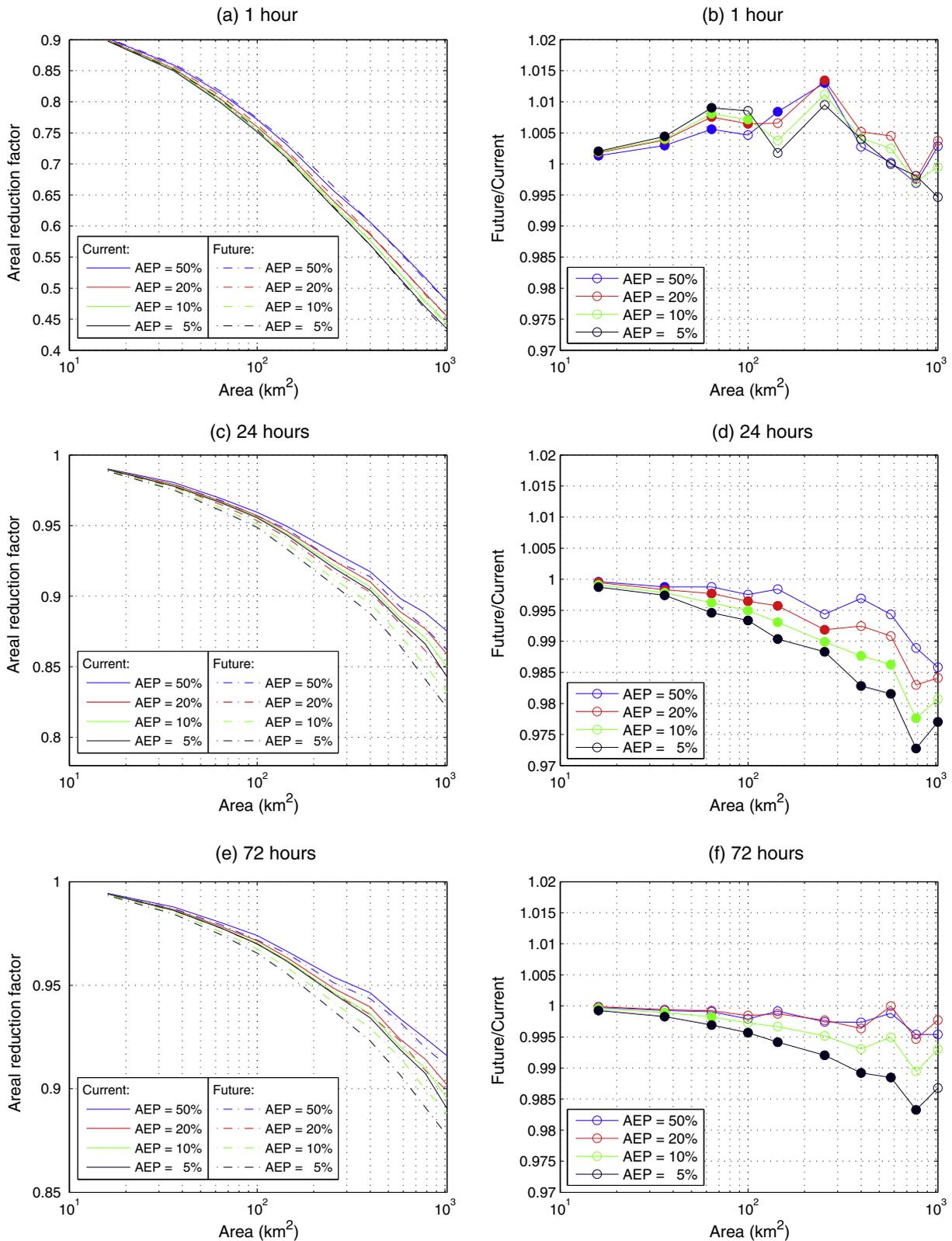
**Fig. 8.** ARFs estimated from WRF/MK3.5 simulations for the current climate (1990–2009, solid curves) and future climate (2040–2059, dashed curves) for storms with AEP from 50% to 5% for storm duration of (a) 1 h, (c) 24 h and (e) 72 h. The ratio of ARFs for the future climate to the current climate is shown in (b) 1 h, (d) 24 h and (f) 72 h. The filled circle indicates where the change of ARFs is significant at 5% level detected by Wilcoxon–Mann–Whitney test.
