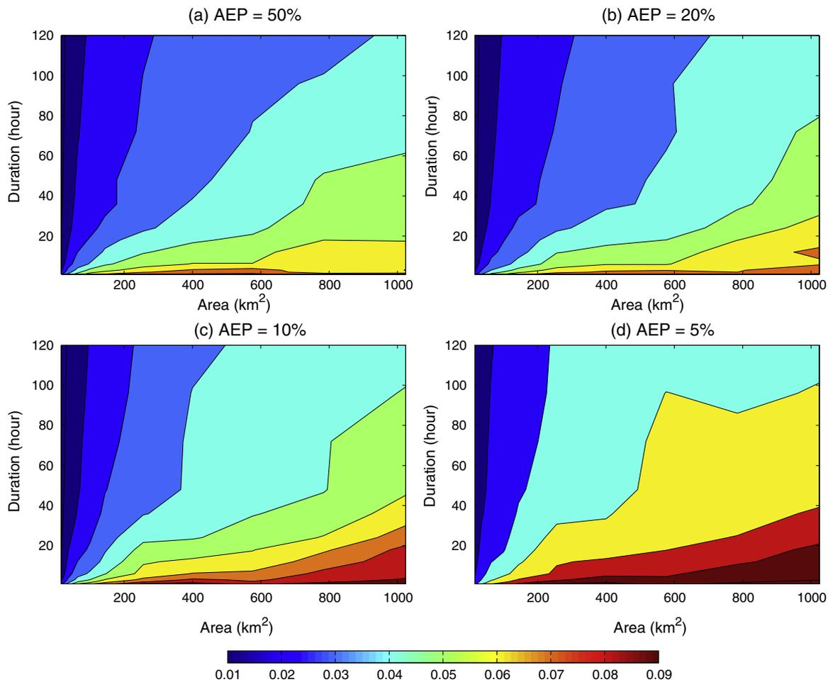
**Fig. 9.** The coefficients of variation (CVs) of the ratios of ARFs derived from WRF/CSIRO MK3.5 for the future climate (2040–2059) to the present climate (1990–2009) for (a) AEP = 50%, (b) AEP = 20%, (c) AEP = 10% and (d) AEP = 5% .
